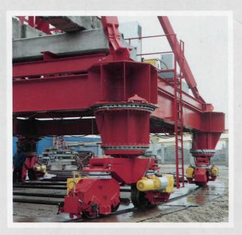
TELESCOPING EQUIPMENT is used when a crane is increased in its height-under-hook by inserting extra mast sections, as a building progresses, or it can be used on initial erection to take a crane to its full height. The equipment can be removed after use. Wall tie frames are also supplied. Climbing and telescoping are carried out hydraulically using fail-safe equipment.
