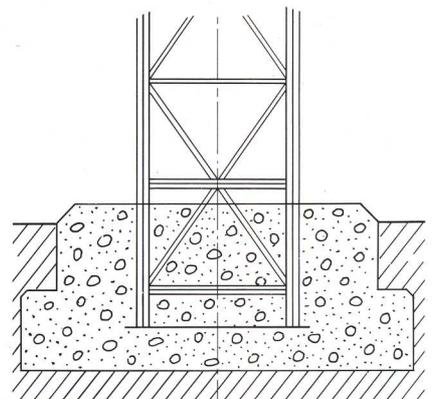
a - ANCRAGE BÉTON POUR GRUE FIXE
